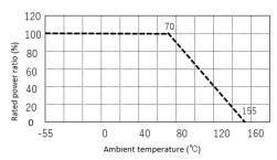
\* Rated power of the resistor is the maximum power which can be loaded continuously at the ambient temperature of 70 °C. For the ambient temperature above 70°C, please use according to the load derating curve (dotted line).
