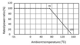
\*Rated power of the resistor is the maximum power which can be loaded continuously at the ambient temperature of 70 °C. For the ambient temperature above 70 °C, please use according to the load derating curve (dotted line). Please note that the component surface temperature does not exceed operating temperature range.
