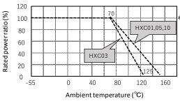
\* Rated power of the resistor is the maximum power which can be loaded continuously at the ambient temperature of 70 °C. For the ambient temperature above 70 °C, please use according to the load derating curve (dotted line). Please note that the component surface temperature does not exceed operating temperature range.
