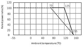
\*Rated power of the resistor is the maximum power which can be loaded continuously at the ambient temperature of 70 °C. For the ambient temperature above 70 °C, please use according to the load derating curve (dotted line). Please note that the component surface temperature does not exceed operating temperature range. \*If the component temperature is below 155°C,
